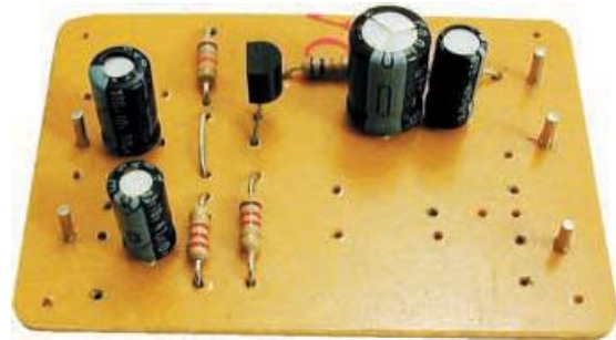
Low Input Impedance Pre-amplifier components mounted on the "single" p.c.b.
