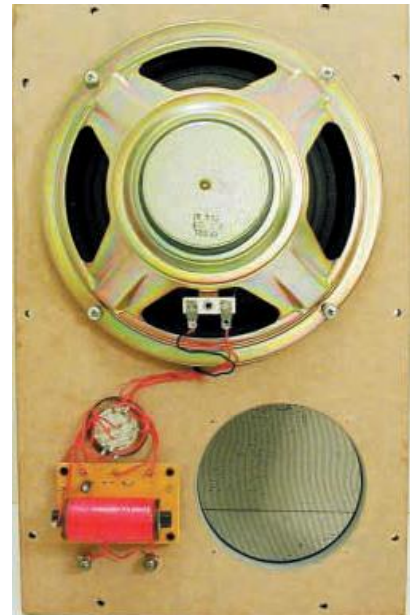
Main speaker and crossover filter (last month) mounted on the rear of the enclosure front panel.
