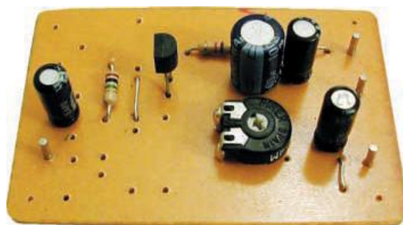
Medium Input Impedance preamplifier components mounted on the "single" p.c.b.
