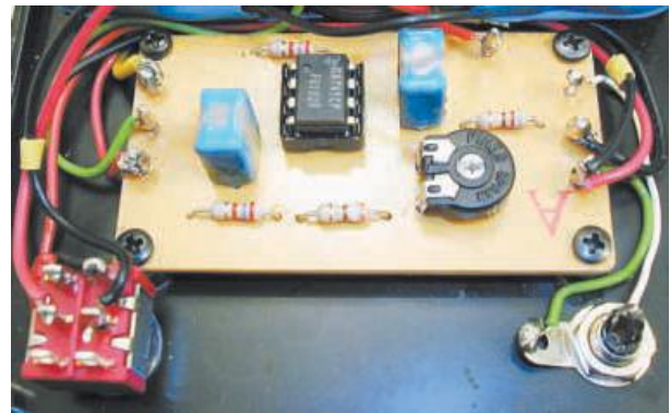
Component layout on the completed circuit board.
