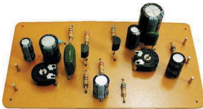
Completed p.c.b. for the Low Noise Preamplifier.
