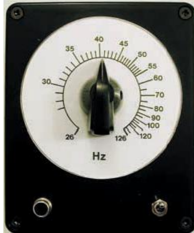
Low Frequency Oscillator for loud speaker resonance checking.
