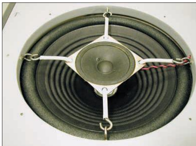
Using cut-down curtain wire, hooks and eyes to suspend the treble speaker over the bass speaker.
