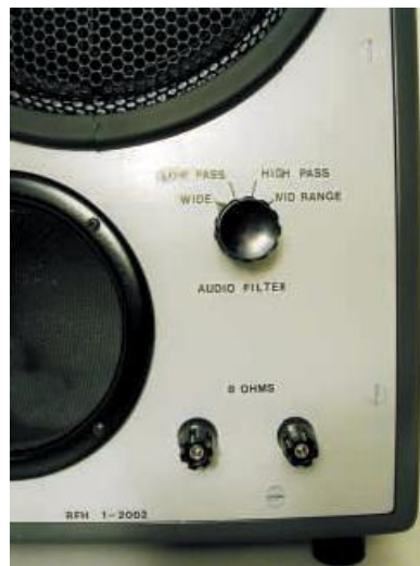
Crossover/Audio Filter selection switch and amplifier input terminals.
